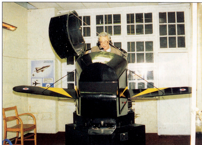
ABOVE Ken Whiffin gives the D-2 at Manston a test flight. The D-2 was introduced in 1942, chiefly for British use, and was an improvement over the D-1 in having a wind-drift mechanism fitted.
